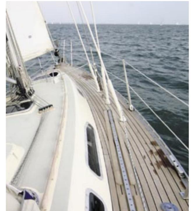
Moving forward is made easy by wide side decks and chunky handrails. Strips of teak edge the genoa tracks to reduce tripping and stubbed toes
